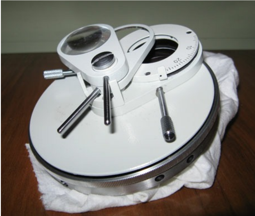
Figure 8 (left bottom): A swing-out filter holder and collector lens completes the package.
