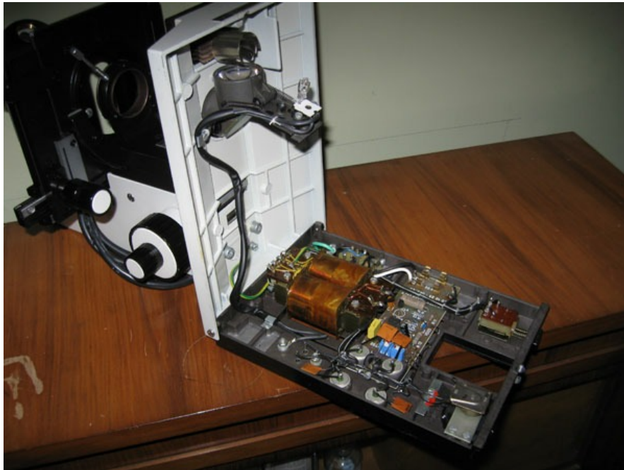
Figure 9 (left top): Access to the electronics is easy by undoing one captured screw and tilting out the hinged base.
