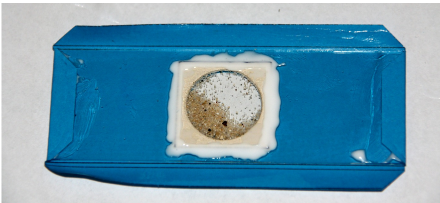
Figure 11: The sand sample is placed into the spacer and a cover glass (difficult to see) is glued on using the same white glue. No mounting medium was applied here, the sand is “air-mounted”. I used quite a lot of glue to seal off everything. The glue will shrink quite a lot as it dries, and will also become transparent.
