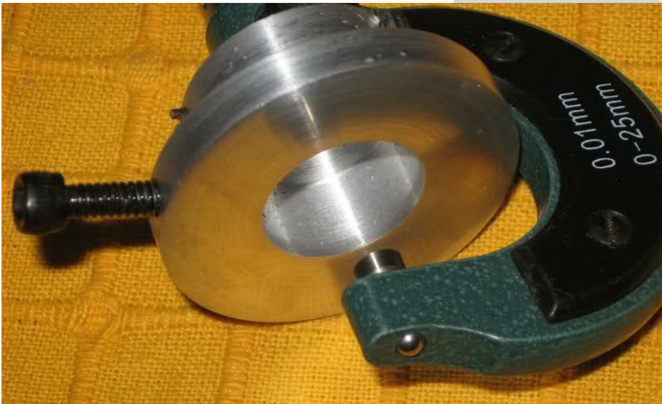
Figure 4: Enlarged view of the finished microtome.
