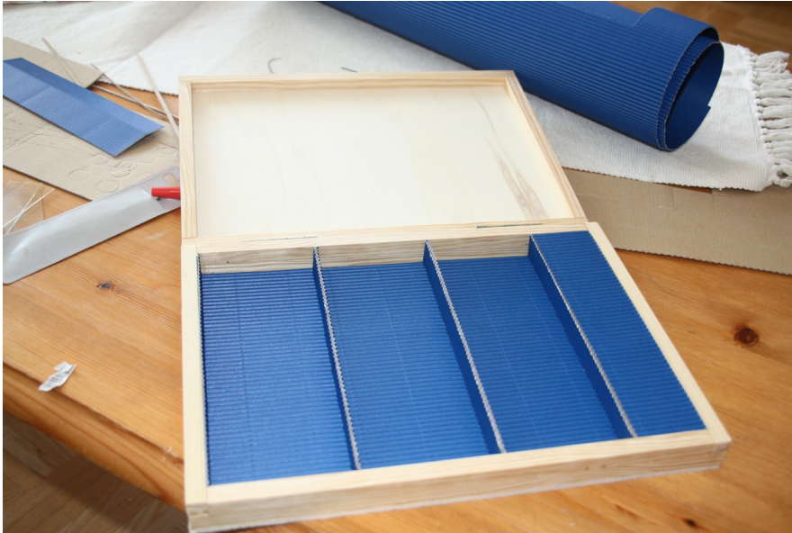
Figure 10: The nearly finished slide box. The box is able to hold 159 slides, 53 for each column.
