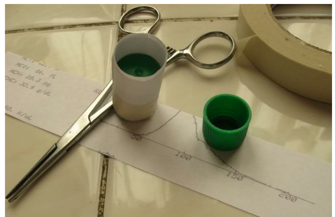
Figure 8 (bottom right): Making the mold out of a cap and paper strips.
