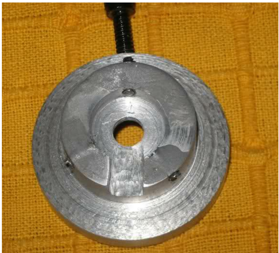
Figure 2 (bottom): The machined part, seen from the bottom, serves as the guide for the microtome knife.
