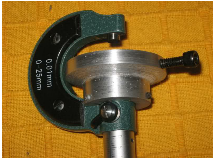
Figure 3: Side view of the finished microtome.
