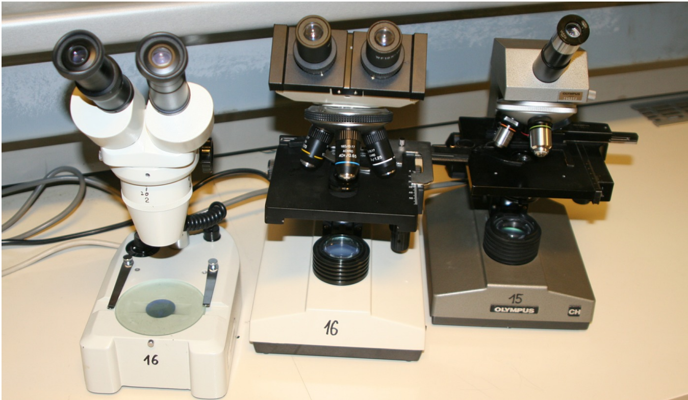
Left: stereo microscope. These are useful for observing opaque objects at low magnification with a stereoscopic view. Center and right: These are both compound microscopes, the middle one with a binocular head. It is not possible to see stereoscopic images with these, even if a binocular head is present. Compound microscopes provide a higher magnification but do not allow for the observation of opaque objects.
