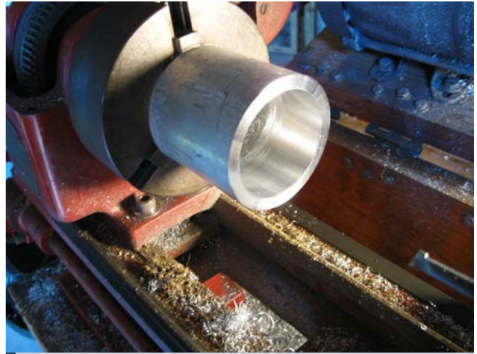
Fig. 15: The inner bearing was cut from aluminum pipe.
