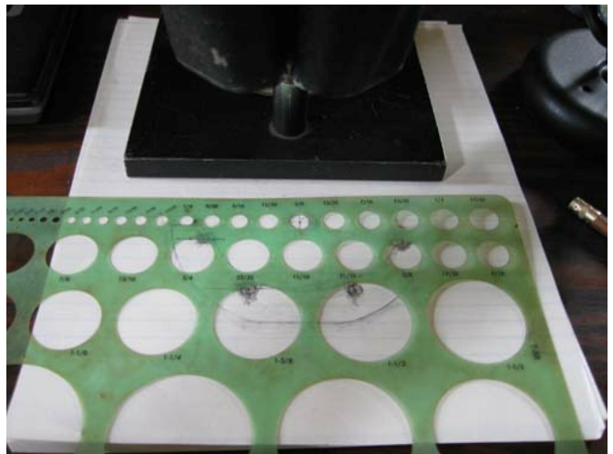
Fig. 11: Finding the center of each hole.
