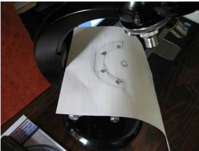
Fig. 10: Transferring the mounting hole pattern of the stage holder to paper.
