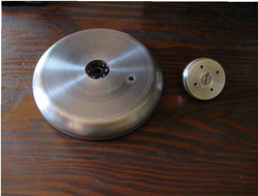
Fig. 4 and 5: The arm interface. I took a 3" diameter "plug" cut with a hole saw from a 1" thick piece of aluminum plate.
