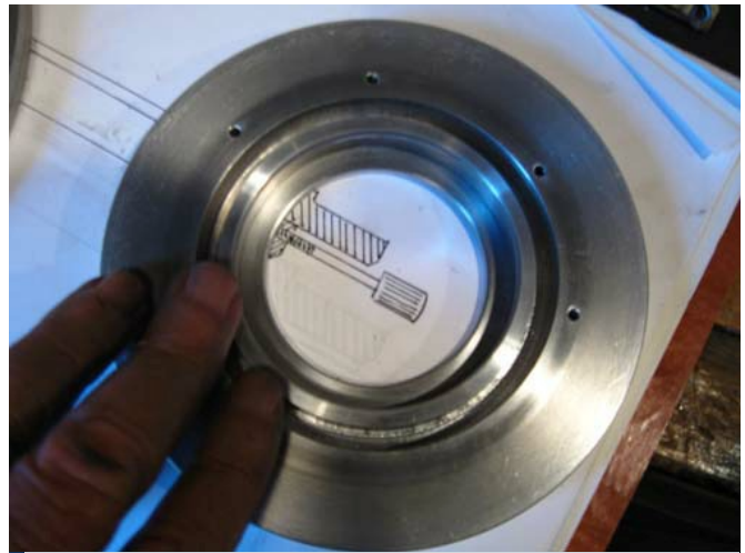
Fig. 17: The holes for mounting the stage are clearly visible.
