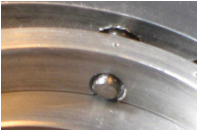
Fig 19-21: Adjusting screws and centering pin.
