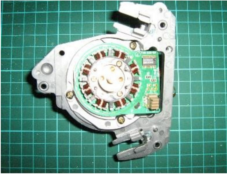
Fig. 3 (top): Rotor with flywheel removed Fig. 4 (bottom): Disassembled rotor
