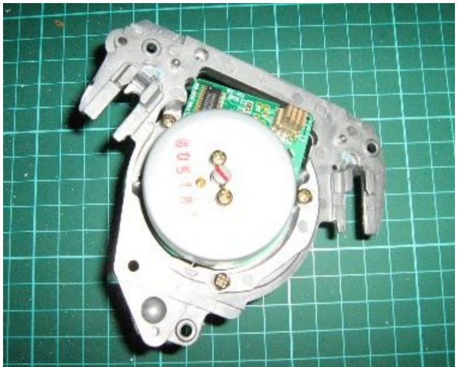
Fig. 1 (top): VCR rotor top view Fig. 2 (bottom): VCR rotor bottom view
