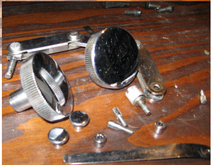
Fig. 2A, 3A. Finally the light was disassembled and cleaned and all the chrome knobs clips etc were soaked in a weak commercial solution (Foz or Ospho) of phosphoric acid for an hour.
