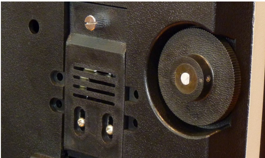
Top: "D" rotary shaft of original potentiometer. Middle: the 1 K Ohm potentiometer mounted to the to the microscope base at the same position of original potentiometer. The 100 Ohm limiting current resistor is soldered to one leg of the potentiometer as show in the picture. Bottom: The dimmer dial mounted in place.
