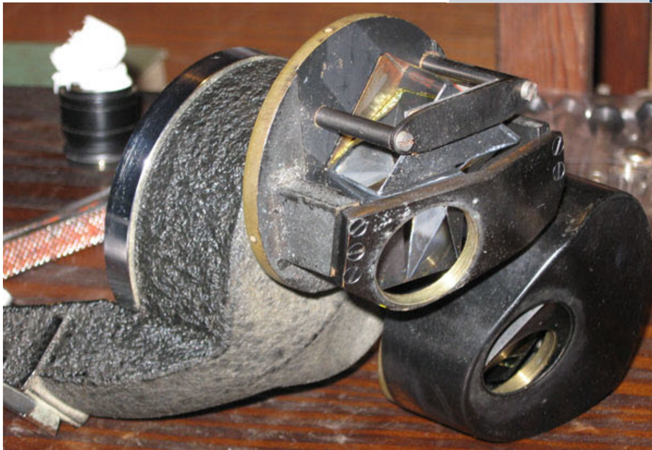
Fig 1A. Notice the very secure top mounting strap on the prism and the multiple screws on either end of the “bridge” that the eyepiece tube screws into. These appear to perhaps be part of the collimation adjustments for the eyepiece tubes (?) as the prisms are cemented together, probably in a jig.
