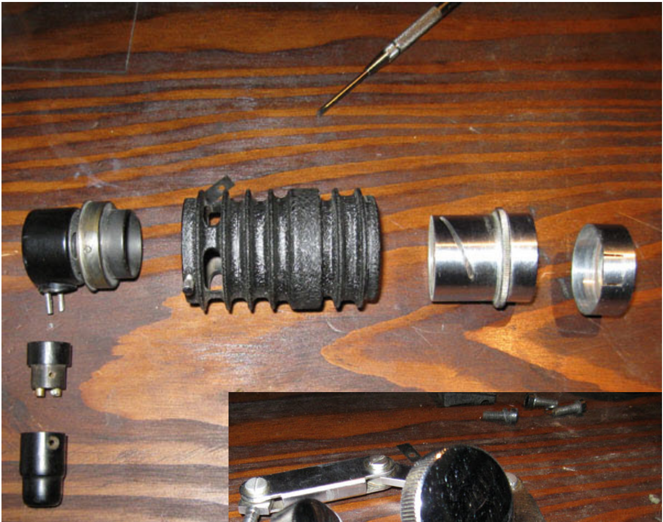
Fig. 2A, 3A. Finally the light was disassembled and cleaned and all the chrome knobs clips etc were soaked in a weak commercial solution (Foz or Ospho) of phosphoric acid for an hour.
