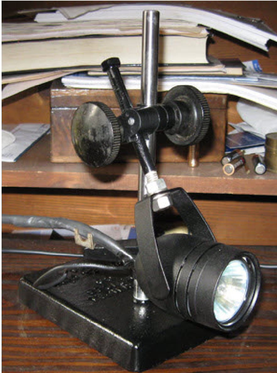
Fig 5A. This light took about 30 minutes to assemble from a $5 pawnshop tool stand and a “salvaged from I can’t remember where” 100W track light.
