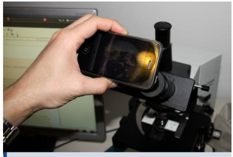
Finding the correct distance to the eye piece is critical for obtaining a vignetting-free image. It may helpful to hold the iPhone with two hands and then release the shutter by using the thumb of the left hand. I found it also useful to rest the left hand against the left eyepiece to obtain a steady image.
