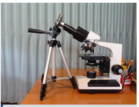
The complete set-up. The tripod is adjusted so that the camera's optics can be fully extended. The camera has to be in line with the eyepiece.
