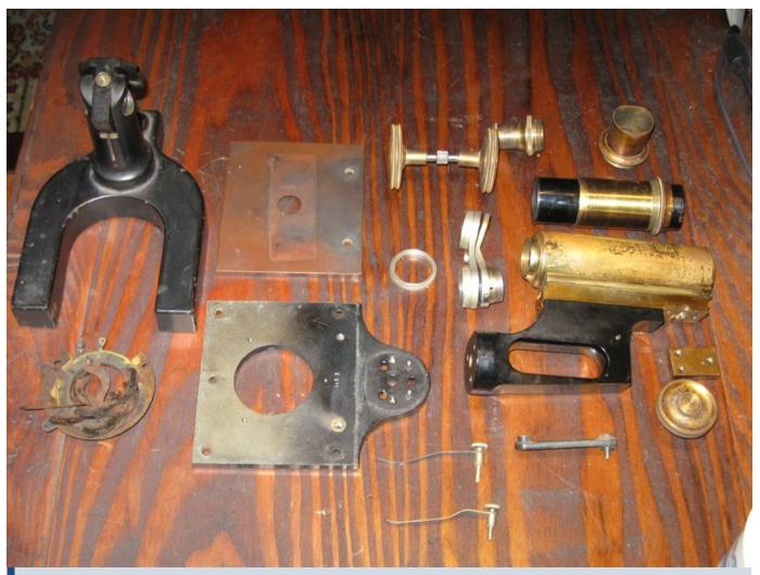
Fig. 1 - Bausch & Lomb BH "Jug Handle" stand disassembled for restoration. The SN indicates 1907 as the year of manufacture. The fact that it has no eyepiece, the eyepiece tube and coarse focus pinion axle are both bent, there is no mirror, an irreparably damaged stage iris and bent nosepiece turret are not insurmountable obstacles to the application I now have planned for this apparatus. "Stay tuned" as they say. Price with shipping was \$16.50.
