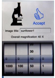
Selecting magnification: After having taken the photograph, the user has to enter the overall magnification (objective x eyepiece) and an image title. The magnification is set by rotating four vertical rolls.
