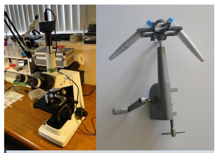
Microscope and centrifuge — two components of a home-lab that complement each other. The hand-centrifuge is able to hold four tubes, only two are shown in the picture. Each plastic tube is held by a metal cylinder. The tubes will swing into a horizontal position.
