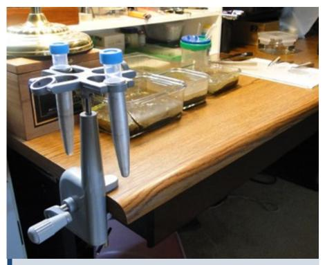
The hand centrifuge can be clamped to a table. Running the centrifuge requires sufficient space. You need spece for operating the crank and for the rotating tubes, which swing into a horizontal position. Make sure that both tubes have the same mass, otherwise the system may start to vibrate. This also increases the wear on the gearing system and may possibly also un-rattle the whole system from the table.
