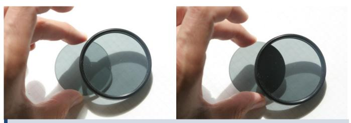
Test the polarizing filters if they are of the correct type. Many polarizing filters that can be bought in photography shops are circular polarizing. These will not work. Place the two filters over each other and rotate one of them. The area where they overlap should be come dark. Just for the fun of it: stick some transparent adhesive tape on a glass slide and place the slide between the two filters. You should see a color play.
